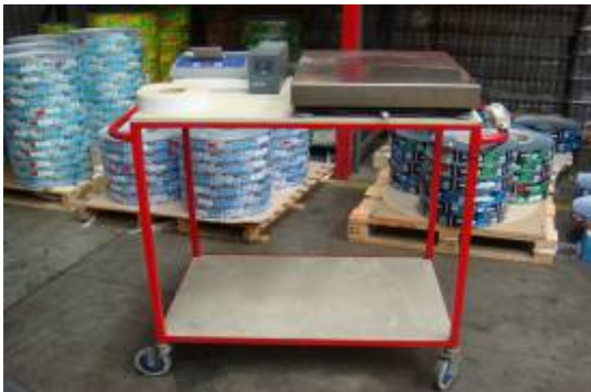
Trolley including digital scales and label printer
